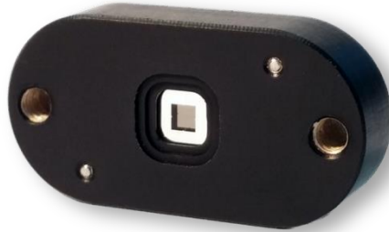
Fig 1. nanoSSOC-A60 sun sensor device
