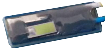
Figure 4 – Example of photodiode soldered onto small PCB
