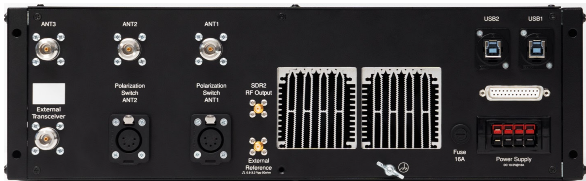
Figure 4 - SDR-Rack back panel
